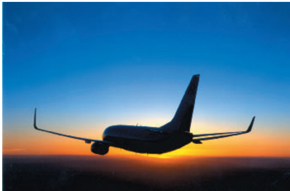
Originally designed for the Gulfstream II, Blended Winglets have become part of the Boeing profile.
